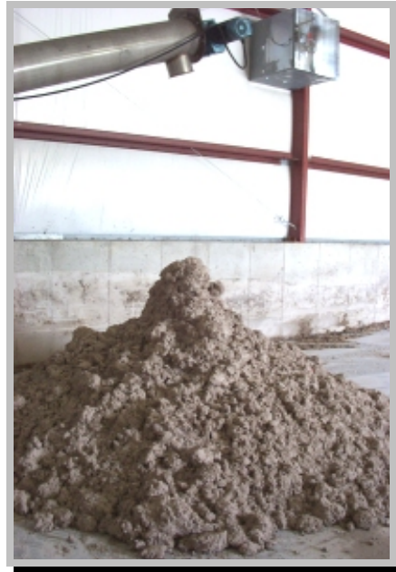
WAS/Lime sludge cake on concrete storage pad at pH10
